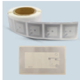
ETS-RT 02A,02B HF Book Tag (13.56 MHz ICODE SLIX2) Size: 80 x 50 / 50 x 50 mm
