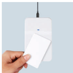
ETC-RD 07 Mifare Card Reader & Writer Interface : USB
